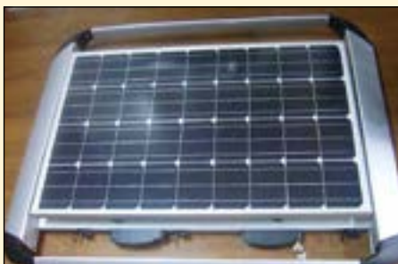
Solar panel to be placed on the cars roof.
